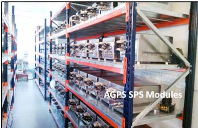
Figure B.2.8 Ion Cyclotron prototype high voltage power supply is successfully commissioned at ITER-India lab; demonstrated for 3MW power with dual output of 27/18kV
