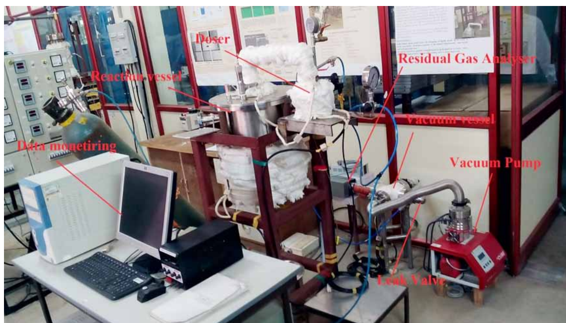
Figure A.2.4.2 Lead-Lithium- water safety experiment set up
