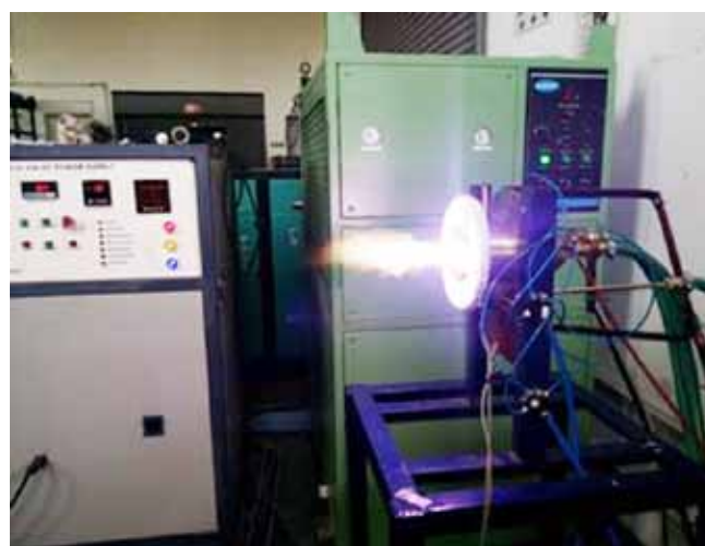
Figure A.3.13.1 atmospheric pressure non-transferred dc plasma torch operating at ~50 kW, along with power supply and heat exchanger
