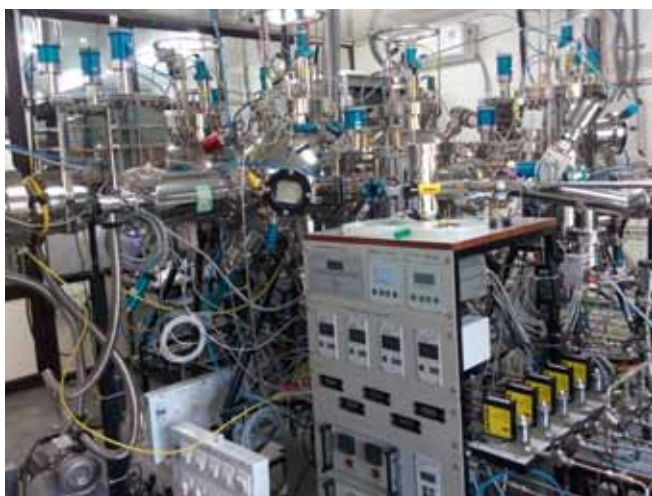
Figure B.1.5 Multi chamber multi magnetron (MCMM) vacuum system installed
