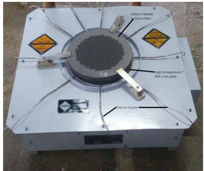
Figure B.2.9 Indigenously developed high temperature (~ 800 °C) blackbody source for calibration of 70 to 1000 GHz
