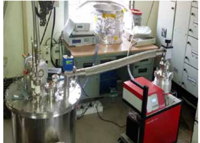
Figure A.2.1.2 Cryogen free facility (Cabling, jacketing and Winding) for manufacturing of superconducting central solenoid are under progress as shown.
