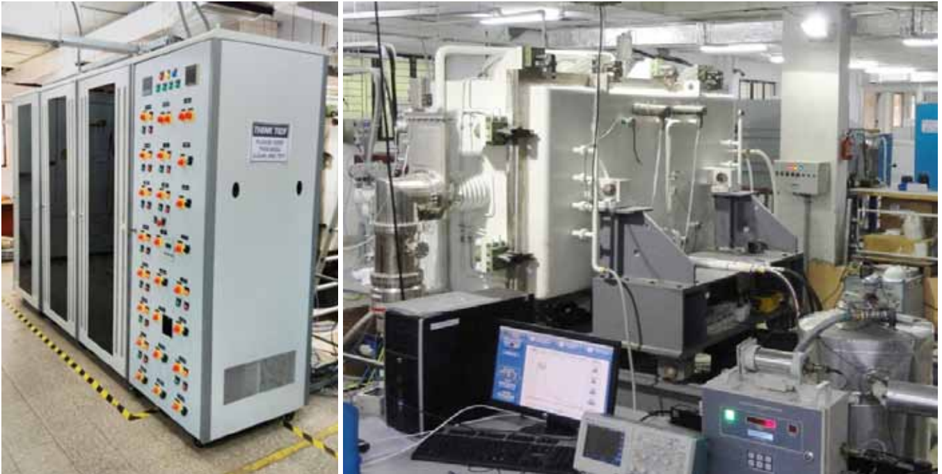
Figure A.2.2.1 Data Acquisition and Control System for High Heat Flux Test Facility
