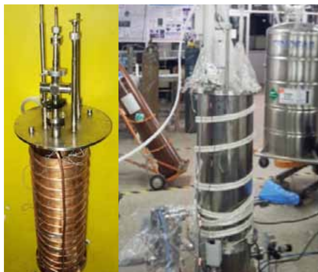
Figure A.2.3.1 Small Scale Cryopumping Facility (SSCF) developed for testing cryo-pump components
