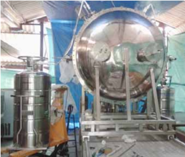
Figure A.2.3.3 Multi Panel Cryopumping Facility
