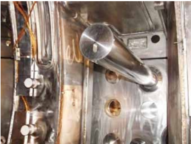
Figure A.1.2.4 Bolometer Camera as seen from inside of the SST-1 vacuum vessel
