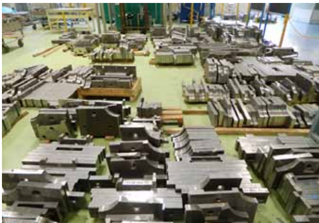
Figure B.2.1 In-Wall Shielding manufactured blocks
