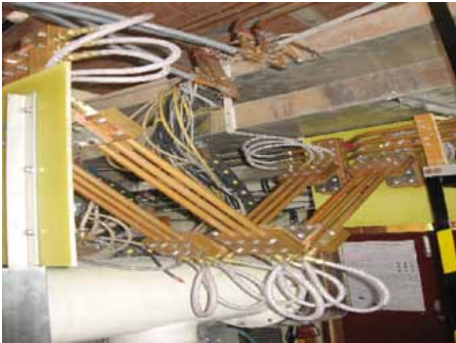
Figure A.3.1.2 Developed high current flexible length feed through. This has an absorption length > 1.2\text{m}
